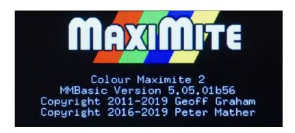
If your monitor remains blank check that you are not still in programming mode (ie, reset the BOOT CONFIG switch or the programming jumper). If you do not have a VGA monitor you can use the serial console (over USB) to check the firmware installation. This is described in the section *Hardware Features* and *Serial Console* in this manual.
