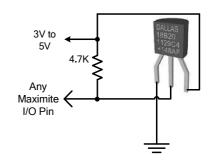
Sensors can also be connected to any of the pins on the eternal I/O connector.
