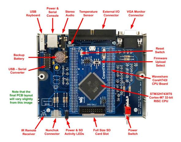
Many suppliers are offering a fully assembled version of this design. These do not use the plug in module concept, instead the ARM Cortex-M7 processor and its supporting components are soldered directly to the main PCB. This makes sense for a machine assembled board and is cheaper to supply.
