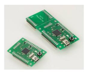
The mini Maximite is a small low cost version of the original (monochrome) Maximite designed for use as an intelligent controller in a user designed system.
