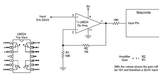
This is a typical arrangement using the popular and inexpensive LM324 quad operational amplifier. The LM324 can operate from a single 5V supply and contains four identical amplifiers in the one 14 pin package. The gain of the amplifier is determined by the ratio of R2 to R1 plus 1 and using the components shown the gain is 101. This number should be used in the BASIC program so that the readings are scaled to represent the input voltage.
