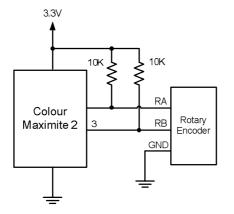
As the knob is turned the rotary encoder will generate a series of signals known as a Gray Code. The program fragment below uses an interrupt to detect and decode the code and update the variable Nbr accordingly.
