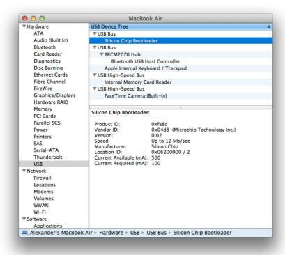
If Maximite is in the bootloader mode ("LOAD FIRMWARE" button was pressed at powering on and the greed LED is now flashing), you should see "Silicon Chip Bootloader" under "USB Bus" on the right.
