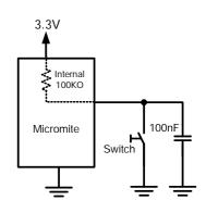
You could check for this in your program, for example by checking 100ms after the first contact closure to confirm that the contacts are indeed closed. A simpler solution is to connect a 100nF capacitor across the switch
