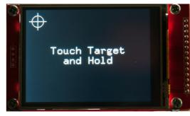
displayed on the console. You also might get a message indicating that the calibration was inaccurate and in that case you should repeat it taking more care to accurately touch the target.
