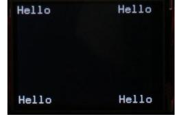
The TEXT command will only display a string, so if you want to display a number (integer or float) you most convert it to a string using the STR\$() function. For example, the following will display 54.7 in the centre of the screen:
