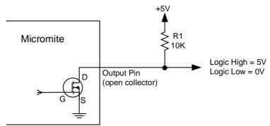
you should use a transistor (either bipolar or FET) to drive the load. To switch 240V AC a more elegant solution is to use a solid state relay. These have full isolation between their input and output and can switch 240V AC loads with a current of up to 10 amps. Some can be directly connected to a Micromite output pin but others need a drive voltage over 4V and in that case you should use an open collector output and a pull up resistor to 5V.
