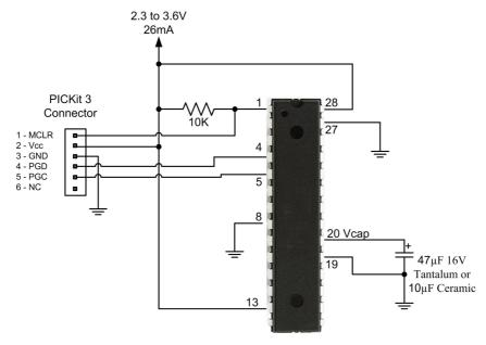
If you are programming the 44-pin module (<u>link</u>) you should plug the PICkit3 onto the six pin programming headers on top of the board. The MPLAB IPE interface is reasonably self explanatory as shown below. This screen shot was taken just after successfully programming the Micromite firmware into a 28-pin Micromite.
