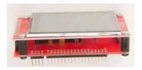
With less than a dozen components the Micromite LCD Backpack can be built in under half an hour.
