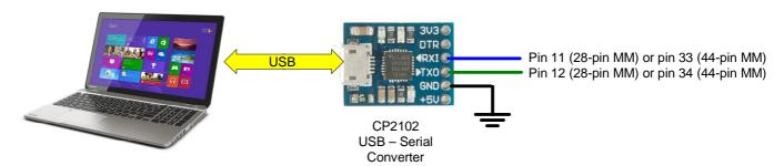
When you plug the USB side of the converter into your computer you may have to load a driver to make it work with the operating system. Once this is done you should note the port number created by your computer for the virtual serial connection. In Windows this can be done by starting Device Manager and checking the "Ports (COM & LPT)" entry for a new COM port as shown on the right.
