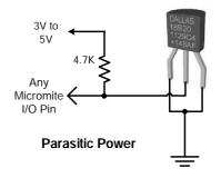
command then later use the TEMPR() function to retrieve the temperature reading. The TEMPR() function will always wait if the sensor is still making the measurement.
