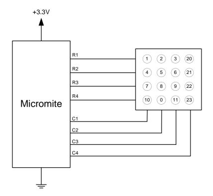
The detection and decoding of key presses is done in the background and the program will continue after this command without interruption. When a key press is detected the value of the variable var will be set to the number representing the key (this is the number inside the circles in the diagram above). Then the interrupt will be called.
