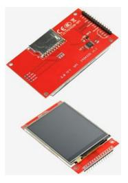
There is a version which uses a TFT panel that requires the colours to be inverted. This is supported by the Micromite by specifying the controller type as ILI9341\_I.
