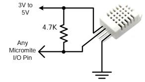
Where 'pin' is the I/O pin to which the sensor is connected. You can use any I/O pin but if the DHT22 is powered from 5V it must be 5V capable. The I/O pin will be automatically configured by MMBasic.
