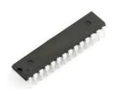
The Micromite is a low cost Microchip PIC32 microcontroller programmed with the MMBasic firmware.
