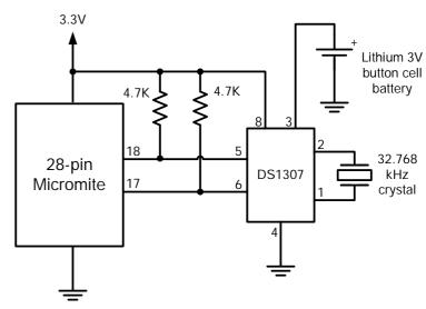
Before you can use the chip its time must be first set. That is done with the RTC SETTIME command which uses the format RTC SETTIME year, month, day, hour, minute, second. Note that the hour must be in 24 hour format.
