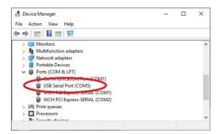
Once this is done you should note the port number created by your computer for the virtual serial connection. In Windows this can be done by starting Device Manager and checking the "Ports (COM & LPT)" entry for a new COM port as shown above.
