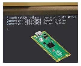
The PicoMiteVGA is a Raspberry Pi Pico running a full featured BASIC interpreter with support for a VGA monitor and a PS2 keyboard for the console input/output.
