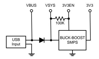
converter will stop switching, internal control circuitry will be turned off, and the load disconnected from the input. You can then power the board via a 3.3V linear regulator feeding into the 3V3 pin. Note that in this case you will still need a 5V supply for the keyboard.
