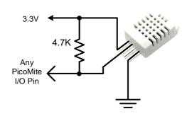
To get the temperature or humidity you use the HUMID command with three arguments as follows: DEVICE HUMID pin, tVar, hVar [,DHT11]
