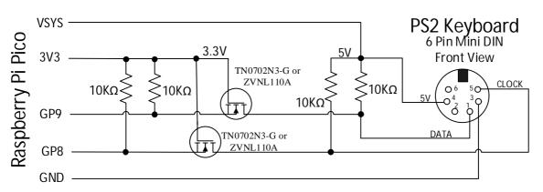
The recommended MOSFET is a TN0702N3-G or ZVNL110A however the commonly available 2N7000 has been tested and also works well.
