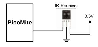
Vishay TSOP4838, Jaycar ZD1952 and Altronics Z1611A. Note that the I/O pins on the PicoMiteVGA are only 3.3V tolerant and so the receiver must be powered by a maximum of 3.3V.
