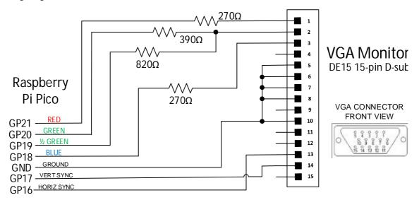
This circuit generates 16 colours in the 4-bit RGB121 format (i.e. 1 bit for red, 2 bits for green, and 1 bit for blue). The output is in the standard VGA format with a pixel rate of 25.175MHz and a frame rate of 60Hz. In monochrome mode the resolution is 640 x 480 however when the colour output is enabled (MODE 2) the pixels are duplicated along both the x and y axis giving a 320 x 240 resolution while the monitor still sees a 640 x 480 signal.
