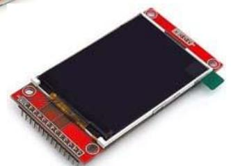
Displays using the ILI9341 controller come in three sizes (2.2, 2.4 and 2.8 inch diagonal measurement) and you can use whatever size that you want although you should be aware that most 2.2 inch displays do not include the touch sensitive screen feature.
