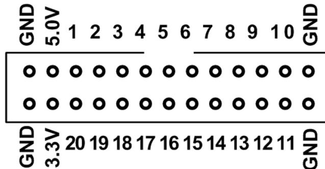
The mini-Maximite also has 20 I/O pins – refer to the board diagram for details.
