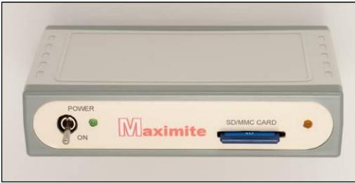
This is the original Maximite computer. It has a monochrome VGA/composite video output and mono sound output.
