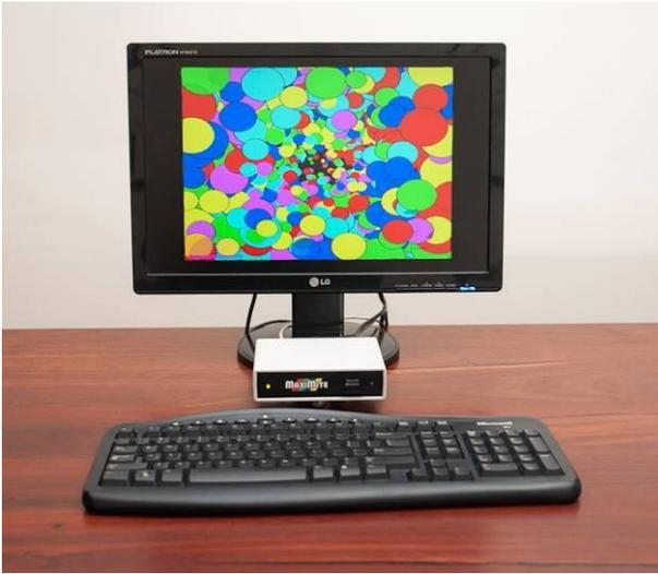
The Colour Maximite is a small and versatile computer running a powerful BASIC interpreter with 128K of working memory.
