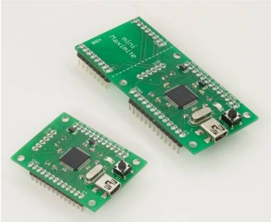
The mini Maximite is a small low cost version of the original (monochrome) Maximite designed for use as an intelligent controller in a user designed system.
