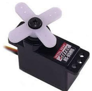
position the rotor at -90°, a pulse width of 2.2ms will position it at +90° and 1.5ms will centre the rotor. These are typical values and can vary between manufacturers.
