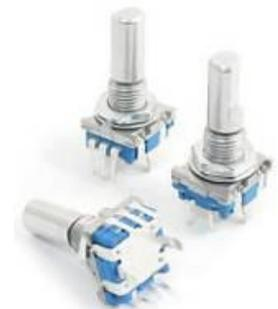
As the knob is turned the rotary encoder will generate a series of signals known as a Gray Code. The program fragment below uses an interrupt to detect and decode the code and update the variable Nbr accordingly.
